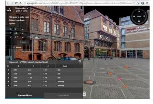
with XYZ coordinates and description in uPANO, and export the feature points list to other applications, such as asset management. If vantage points other than the laser scanner setup positions are desired, customers should use LiDAR2Map, a similar feature on the uGRIDD platform.
